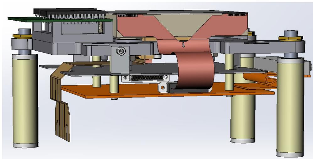
Figure 12. CCD mount assembly containing a CCD231-C6, offset guide and focus detectors, amplifier PCB, and thermal control components.
