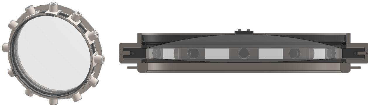
Figure 6. Field lens mechanical assembly in isometric and cross section views, at different scales.
