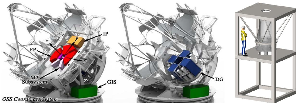
Figure 1. The various GMT instrument ports are shown in the left and middle panels. ComCam, shown at a different scale on the right, will mount at the DG position in its own dedicated IMF.
