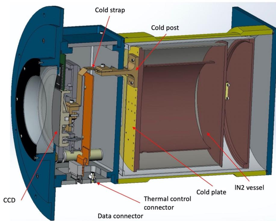
Figure 13. CCD camera in cross-section.
