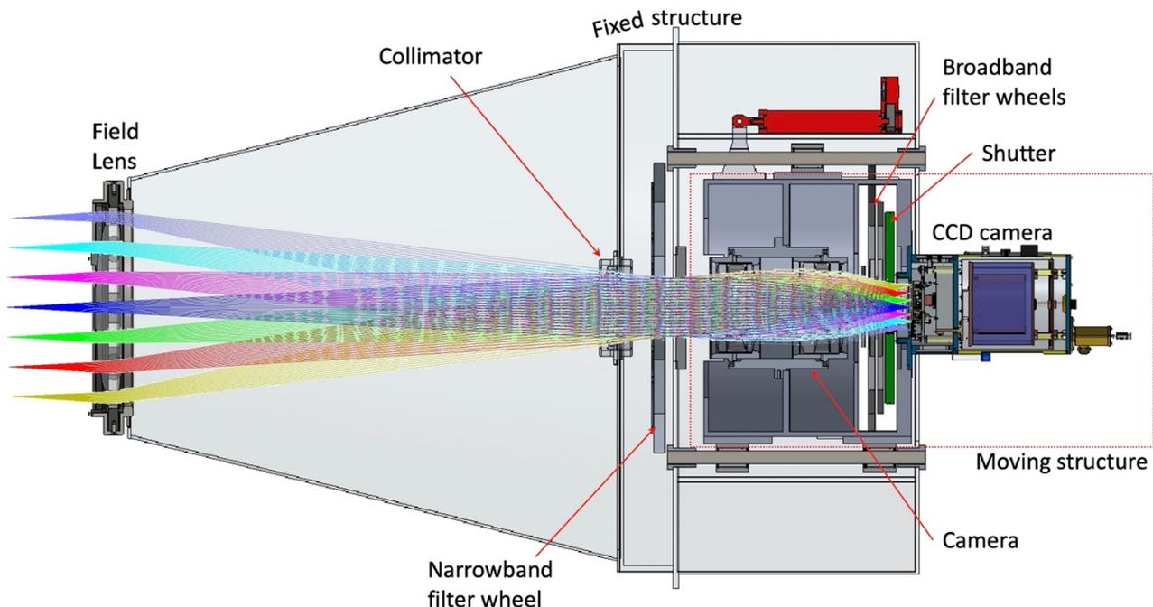
Figure 8. ComCam in cross-section. Light from seven evenly spaced field positions is shown.
