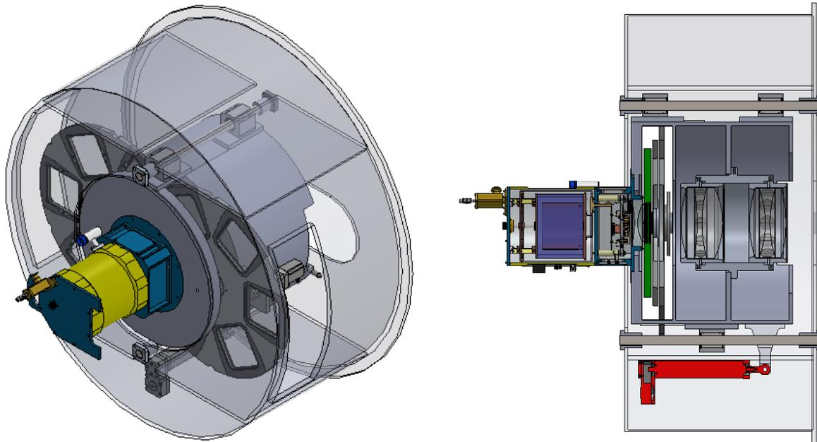
Figure 10. Camera support structure subassembly in isometric and section views. One section of the fixed, main support structure is shown semi-transparent.
