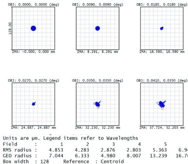
Figure 5. Example spot diagram for  $\lambda 550$  nm in a 0.5 arcsec box. Field positions are shown in Figure 2.
