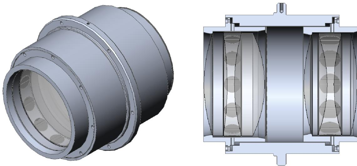
Figure 7. Camera mechanical assembly in isometric and cross section views. The camera triplet lens cells insert into a central barrel. The collimator lens cell is similar in design to the camera lens cells.
