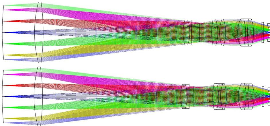
Figure 4. Narrow band filter (top) and Fabry-Perot etalon (bottom) modes.
