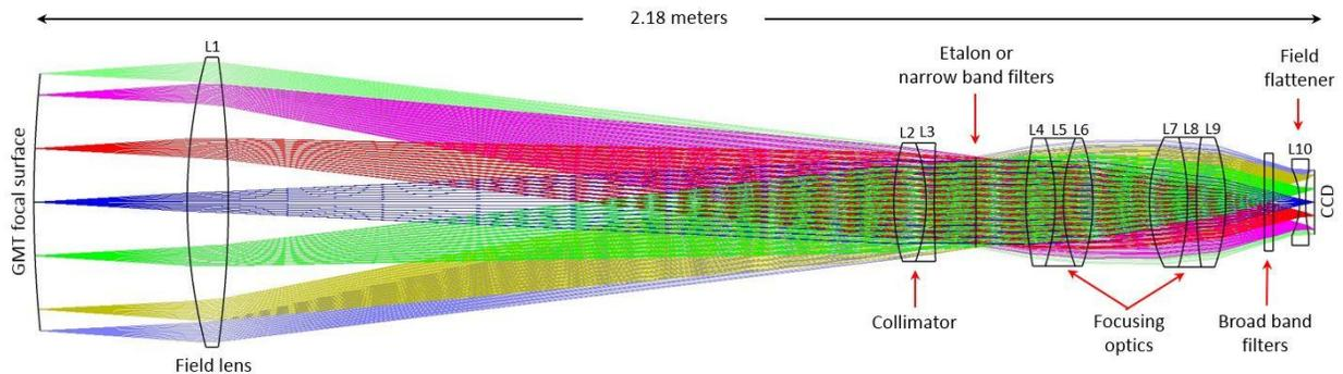
Figure 3. ComCam wideband optical layout.
