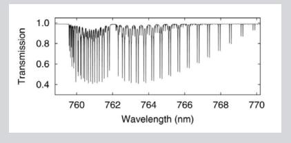
of ~760 nm, showing the most prominent  $O_2$  band. Because the exoplanet system will be moving relative to us, the  $O_2$  lines from the exoplanet will appear Doppler-shifted with respect to the  $O_2$  telluric lines, and we can use that Doppler-shift information and cross-correlation techniques to detect the exoplanet's  $O_2$ . This same technique works in the near-infrared for  $H_2O$ ,  $CO_2$ , or  $CH_4$  with the GMTNIRS instrument (Figure adapted from Rodler & López-Morales 2014).
