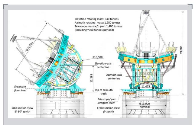
**Figure 1-3** This figure shows a section view of the GMT from the base of the pier (extending below ground level) to the top of the secondary mirror, almost 55 m above the ground. The telescope structure moves in altitude and azimuth, like all modern telescope mounts; however, the structure is unusually compact and stiff for the diameter of the mirror. This enables better resonant performance, lower cross-section to wind, and allows the enclosure to be smaller.
