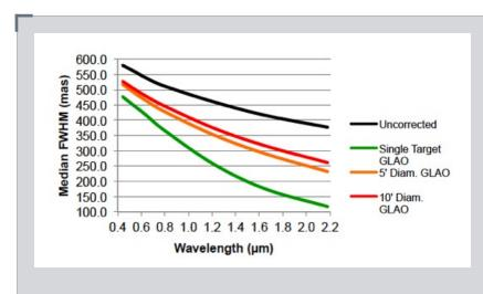
Figure 1-5 Image quality and observing modes: the black line shows the measured diameter of the image size (full width at half maximum, or FWHM) of images taken in natural seeing at Cerro Campanas. The colored lines show the simulated, mean FWHM with ground-layer adaptive optics (GLAO) for three fields of view. Better GLAO correction is obtained for smaller fields of view. These mean values are indicative of a world-class observing site with low atmospheric turbulence.
