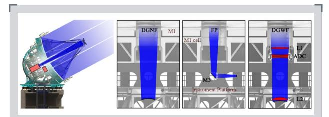
**Figure 1-8** The GMT's light path (in blue) and focal stations. From the left: (1) the complete telescope, (2) the direct Gregorian focus without corrector (Direct Gregorian Narrow Field focus), (3) one of three folded ports (FP), and (4) direct Gregorian focus with the wide field (DGWF) corrector (in red). The gravity invariant stations are not shown.
