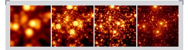
**Figure 1-6** The progression of images from left to right shows the impact of adaptive optics with the GMT: (1) natural seeing at 0.5 arcsecond resolution. (2) Hubble Space Telescope with 0.2 arcsecond resolution. (3) a simulated image with James Webb Space Telescope with 0.07 arcsecond resolution, and (4) a simulation of the 0.02 arcsecond resolution images that the GMT will obtain with natural guide star adaptive optics.
