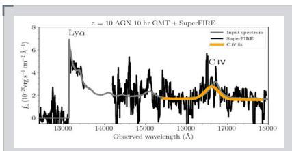
Figure 9-11 The GMT will measure supermassive black hole masses out to  $z \sim 10$  using the kinematics (velocities) of ionized gas as it speeds in orbit around the black hole. Because of the immense gravity of the black hole, the gas swirls at 1000's of km/s. This figure presents a simulation of a SuperFIRE-like instrument on the GMT with a one night (10 hours) observation of a faint ( $H = 26^{th}$  magnitude) AGN at z = 10 (black line), and similar results are possible with integrated
